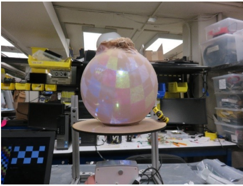
Figure 3: The output of a Asus 600 lumen project and mirror to fill a 10" sphere in ambient light filled room.
