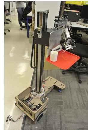
Figure 8: Persona robot with a low cost holonomic mast.
